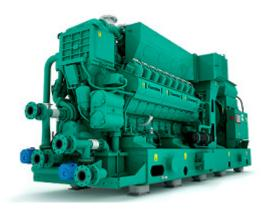
Alternator – Several alternator sizes offer selectable voltage and temperature rise with low reactance 2/3 pitch windings; low waveform distortion with non-linear loads, fault clearing short-circuit capability, class F or H insulation (see Alternator Data Sheet for details), bearing and stator RTDs and anti-condensation heater. Mechanically strengthened for use on utility paralleling with unreliable grid.
